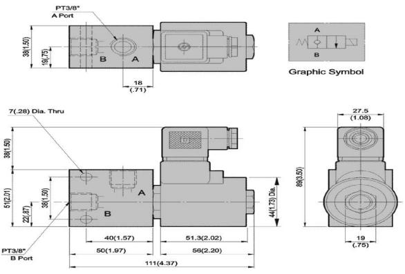
3/4" Line Mounting Solenoid Check Valves
