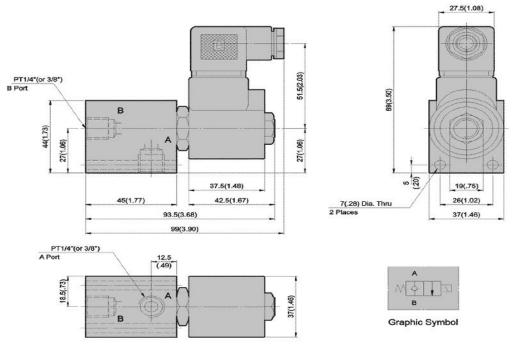
3/8" Line Mounting Solenoid Check Valves
